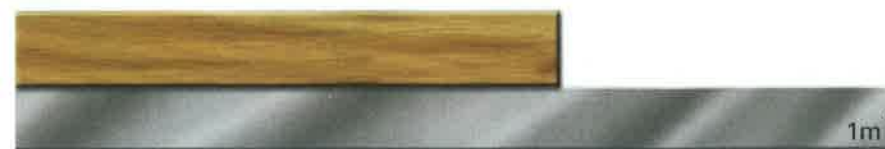
Figure 3.5 Three differently calibrated meter sticks are used to measure the length of a board. a A meter stick calibrated in a 1-m interval. b A meter stick calibrated in 0.1-m intervals. c A meter stick calibrated in 0.01-m intervals. Measuring How many significant figures are reported in each measurement?
