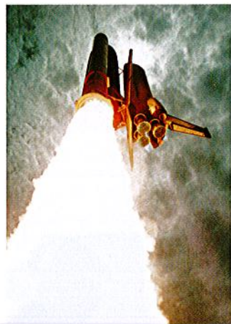
The shuttle launches due to the reaction of \text{H}_2 and \text{O}_2 . The water vapor produced expands rapidly to thrust the shuttle upward.
