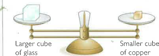
The small cube of copper exactly balances the mass of the larger cube of glass.
