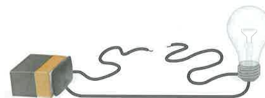
The light bulb doesn't light up because there's a break in the wire.
