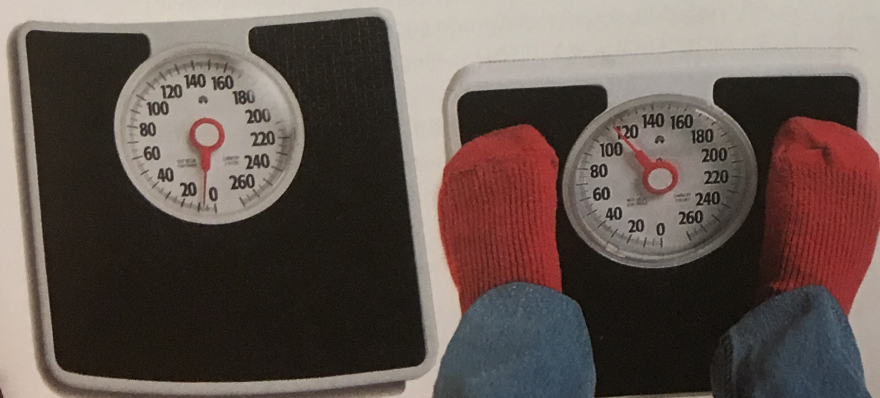
Figure 3.3 The scale below has not been properly zeroed, so the reading obtained for the person's weight is inaccurate. There is a difference between the person's correct weight and the measured value. Calculating What is the percent error of a measured value of 114 lb if the person's actual weight is 107 lb?
